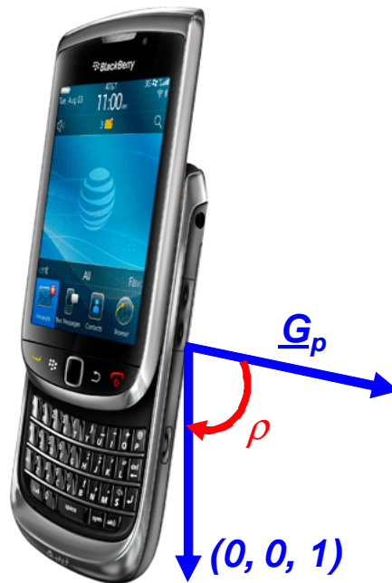
Figure 7. Calculation of the Tilt Angle \rho from Vertical
