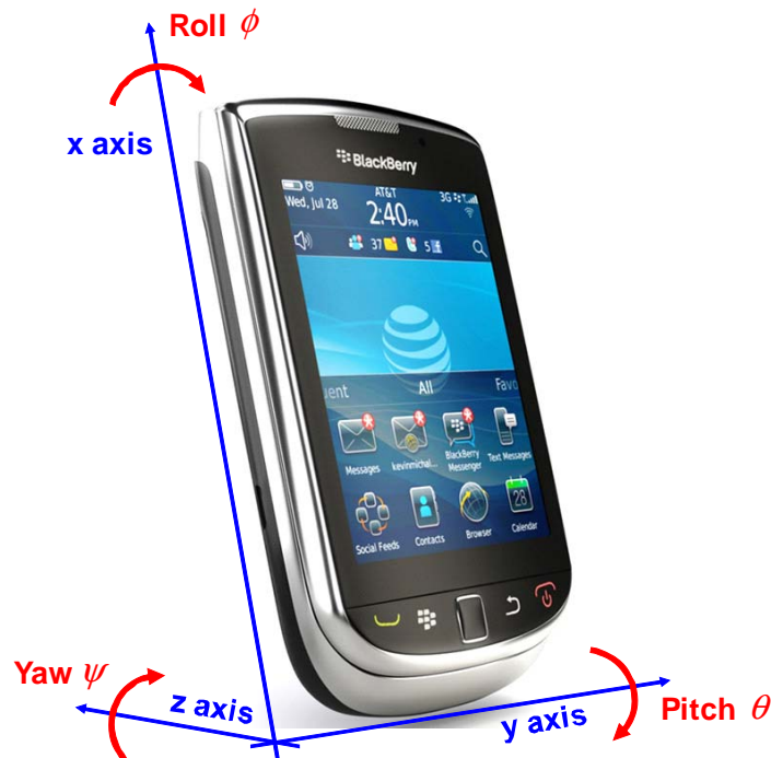
Figure 3. Definition of Coordinate System and Rotation Axes
